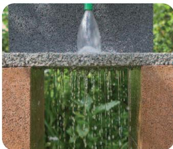
**Porous asphalt** is the same as regular asphalt except it is manufactured with the fine materials omitted, leaving open spaces that allow water to filter through to a “recharge” or drainage bed.
