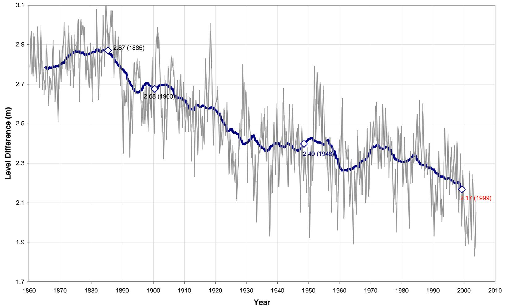
**Figure H Change in Level Difference between Lakes Michigan-Huron and Erie due to Erosion and Man-Made Intervention (seasonal and weather induced changes removed through normalization)**
