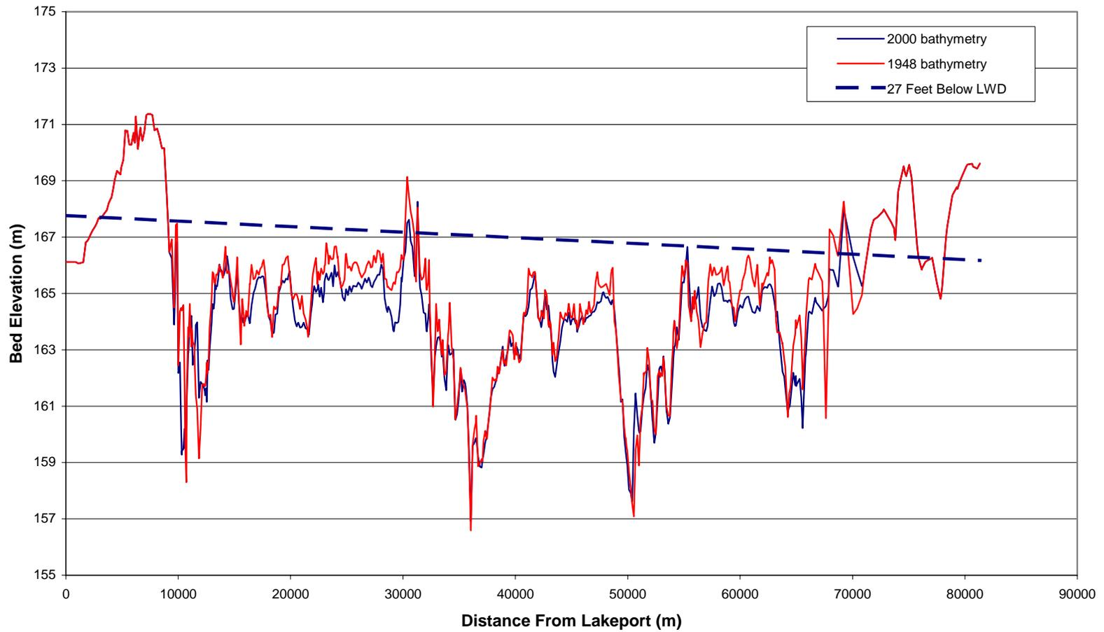
**Figure 5.7 Comparison of Bed Elevation Profiles between 1948 and 2000**
