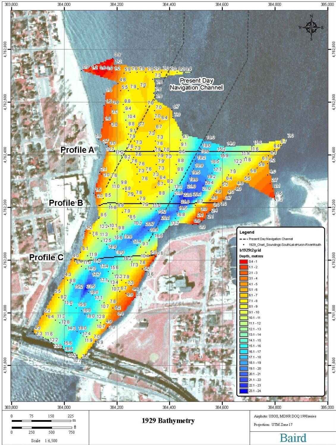
**Figure 3.2 Bathymetry at St. Clair River Inlet in 1929**
