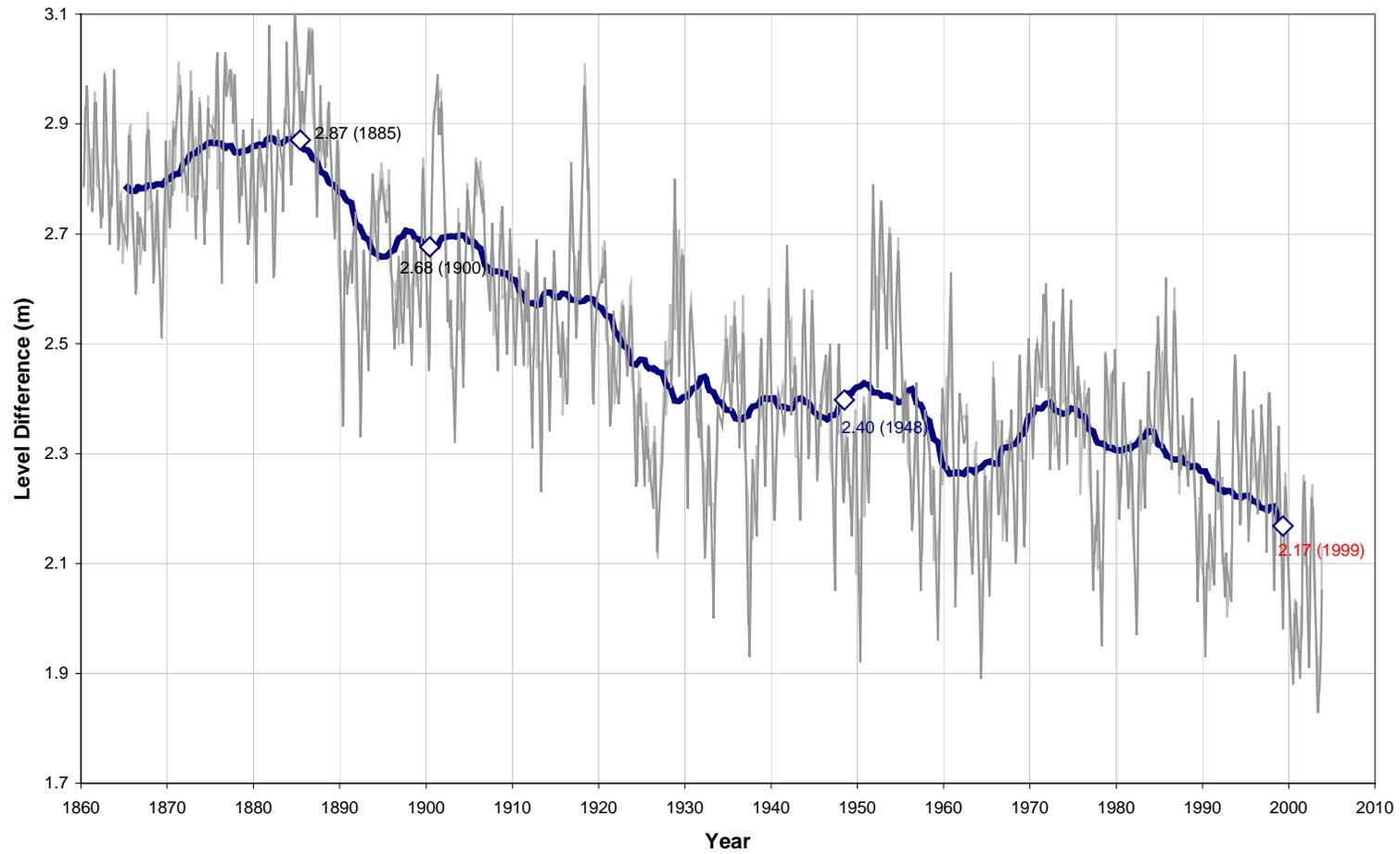
**Figure 6.2** Change in Level Difference between Lakes Michigan-Huron and Erie due to Erosion and Man-Made Intervention (seasonal and weather induced changes removed through normalization)
