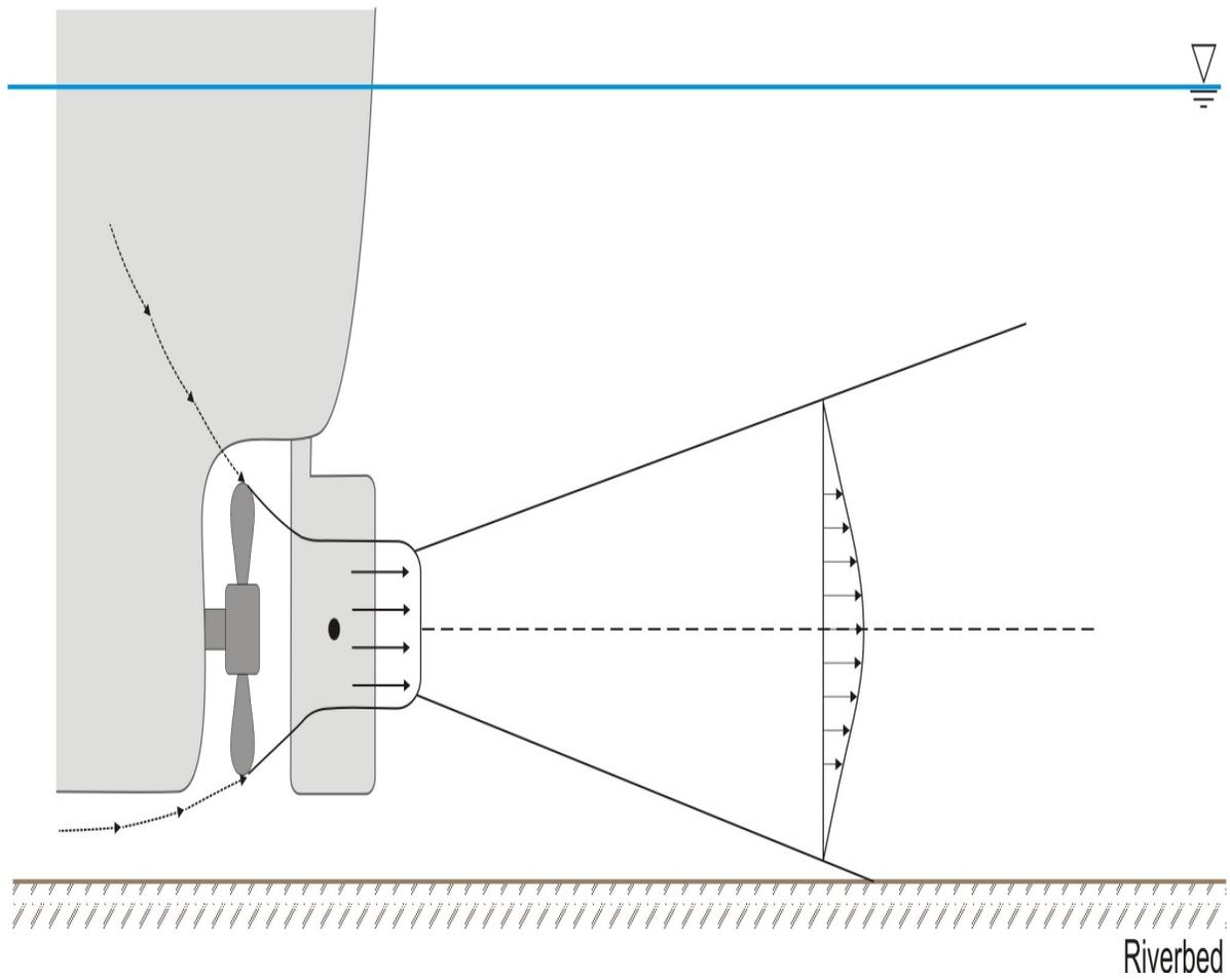
**Figure 7.5 Velocity jet behind vessel.**
