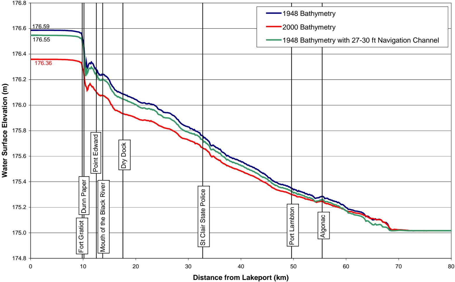
**Figure 5.6 Water Surface Profile showing Head Drop from 1948 to 2000**
