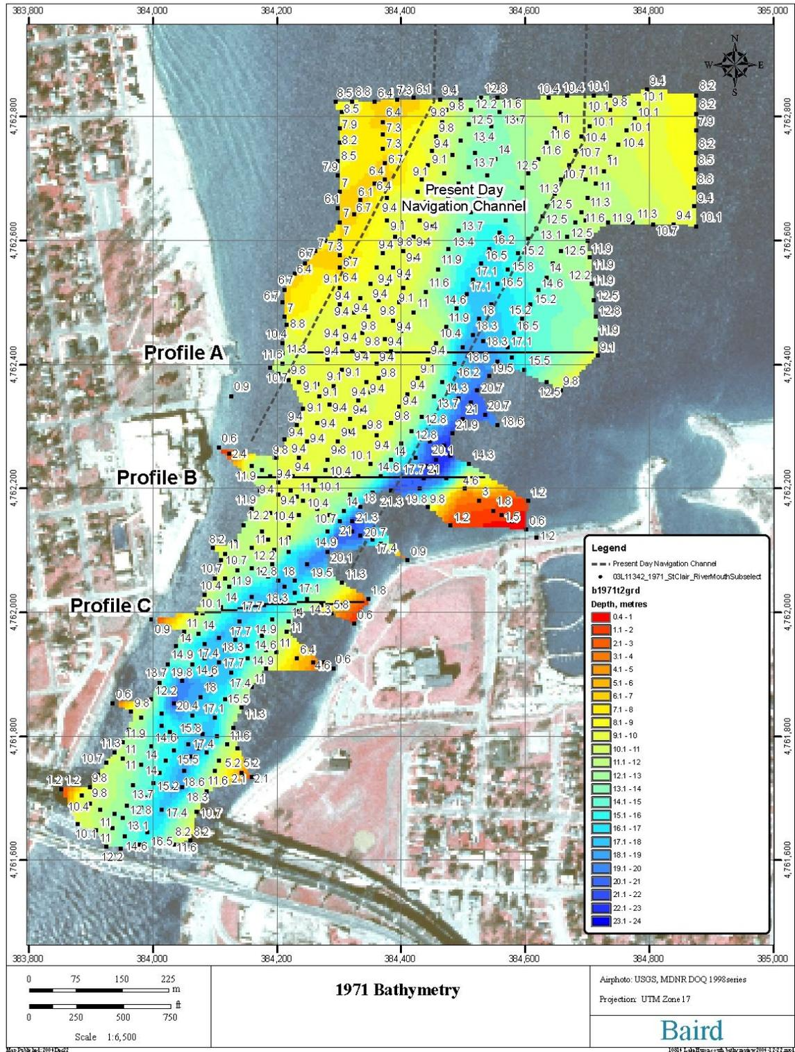
**Figure 3.3 Bathymetry at St. Clair River Inlet in 1971**
