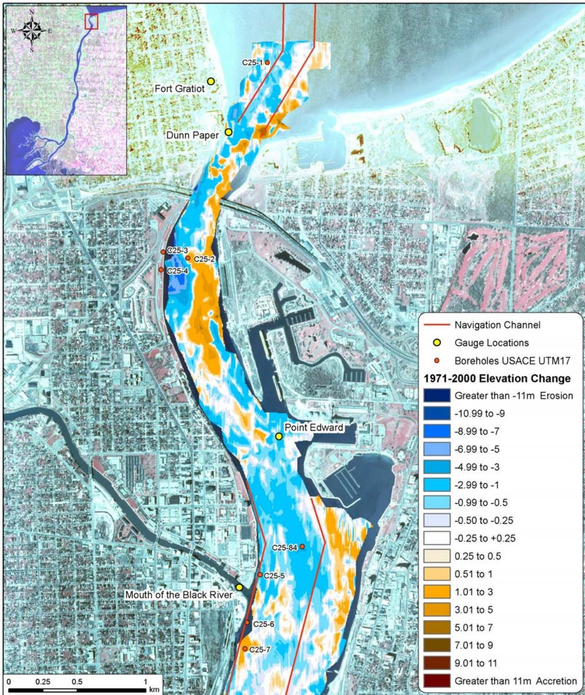
**Figure 4.1 USACE Borehole Data and Erosion/Deposition Areas**
