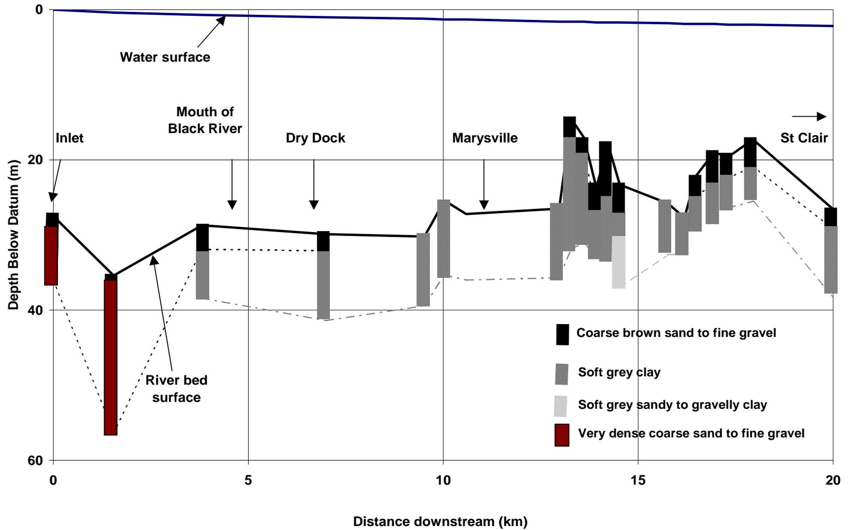
Figure 7.3 Distribution of Bed Materials Along the River based on Borehole Data
