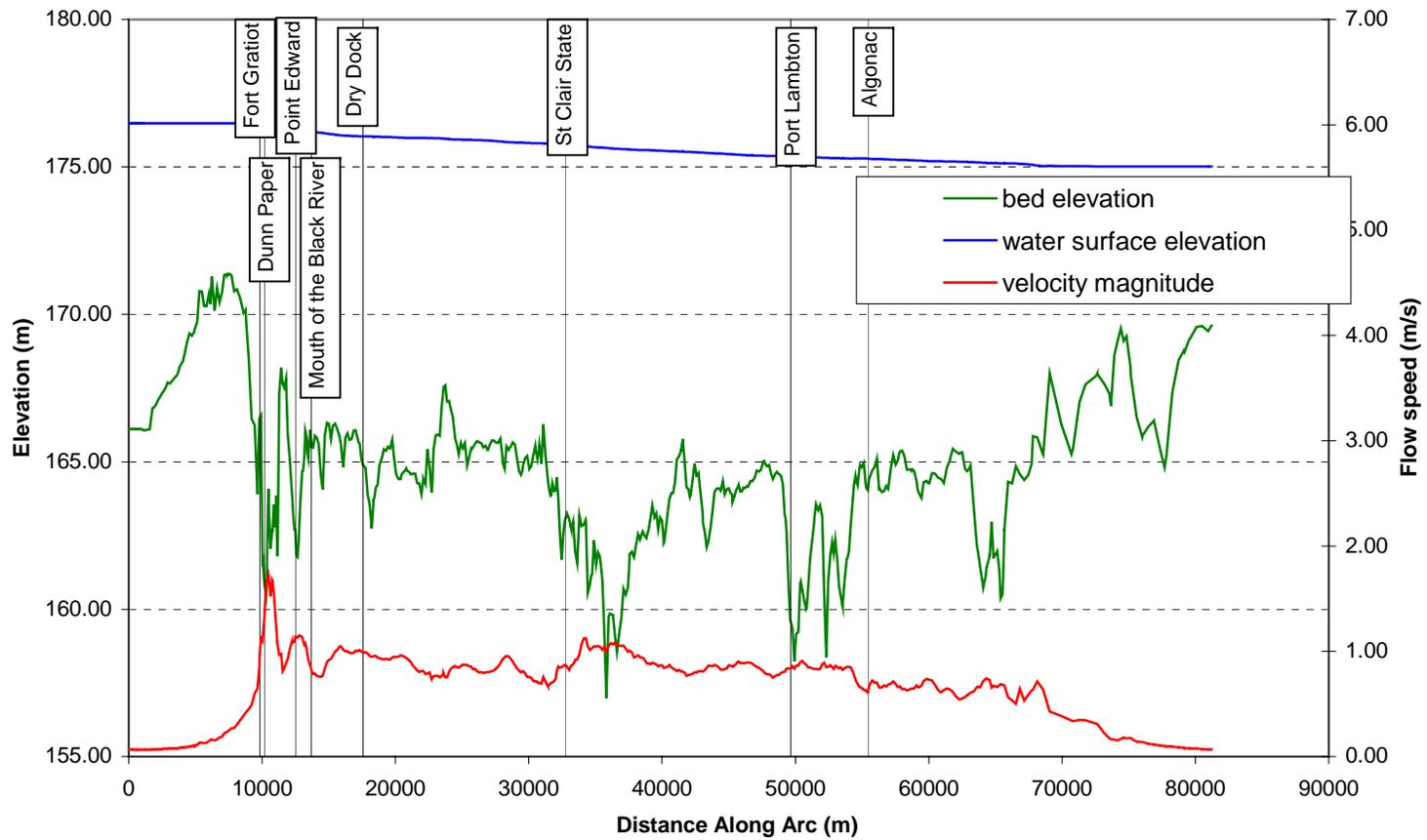
**Figure 5.5 Model Output for 2000 Bathymetry, Flow = 5,200 m<sup>3</sup>/s.**
