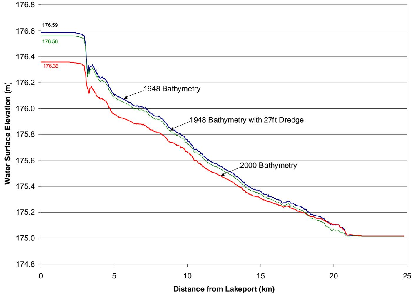
**Figure G Water Surface Profile from the Numerical Model Simulations**
