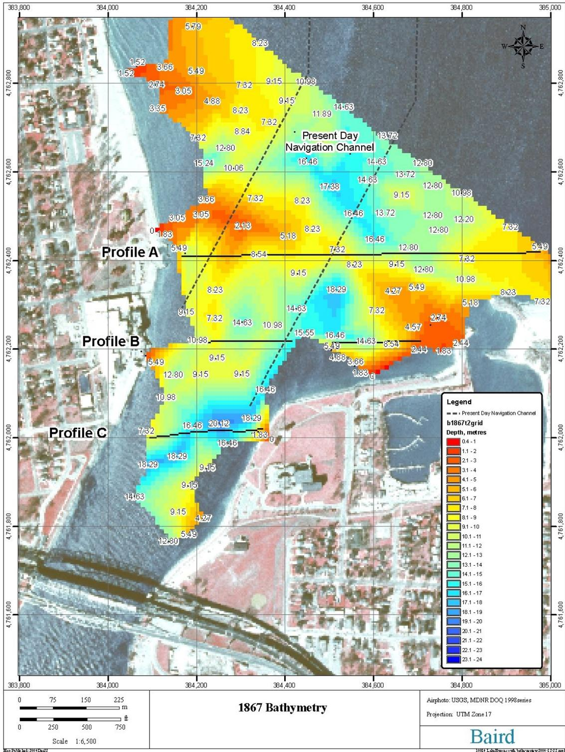
**Figure 3.1 Bathymetry at St. Clair River Inlet in 1867**
