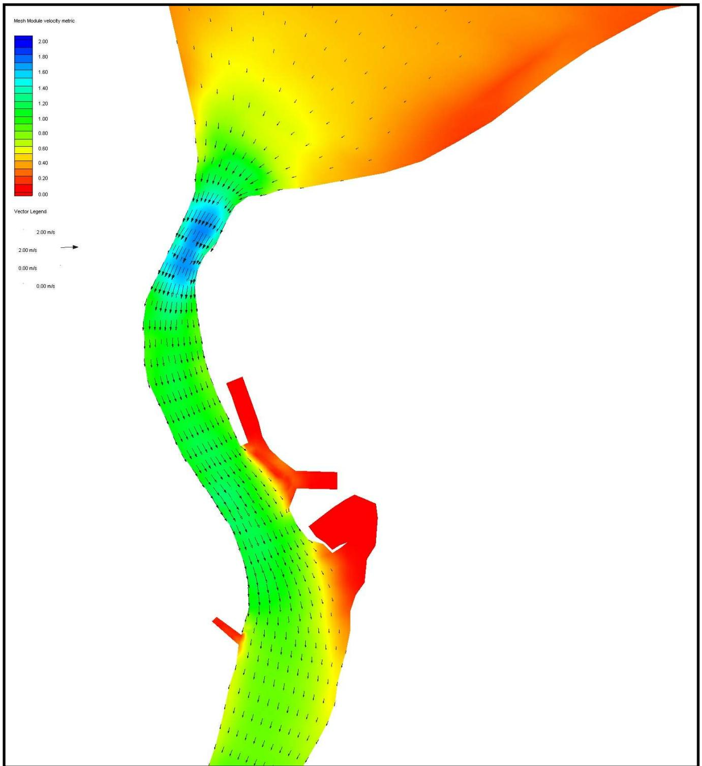
**Figure 5.4 Flow vectors with 2000 Bathymetry**
