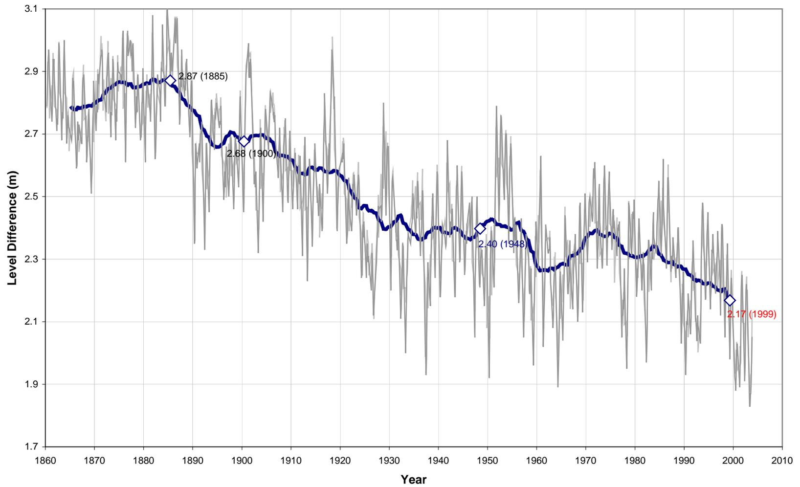
**Figure 1.2 Change in Level Difference between Lakes Michigan-Huron and Erie due to Erosion and Man-Made Intervention**
