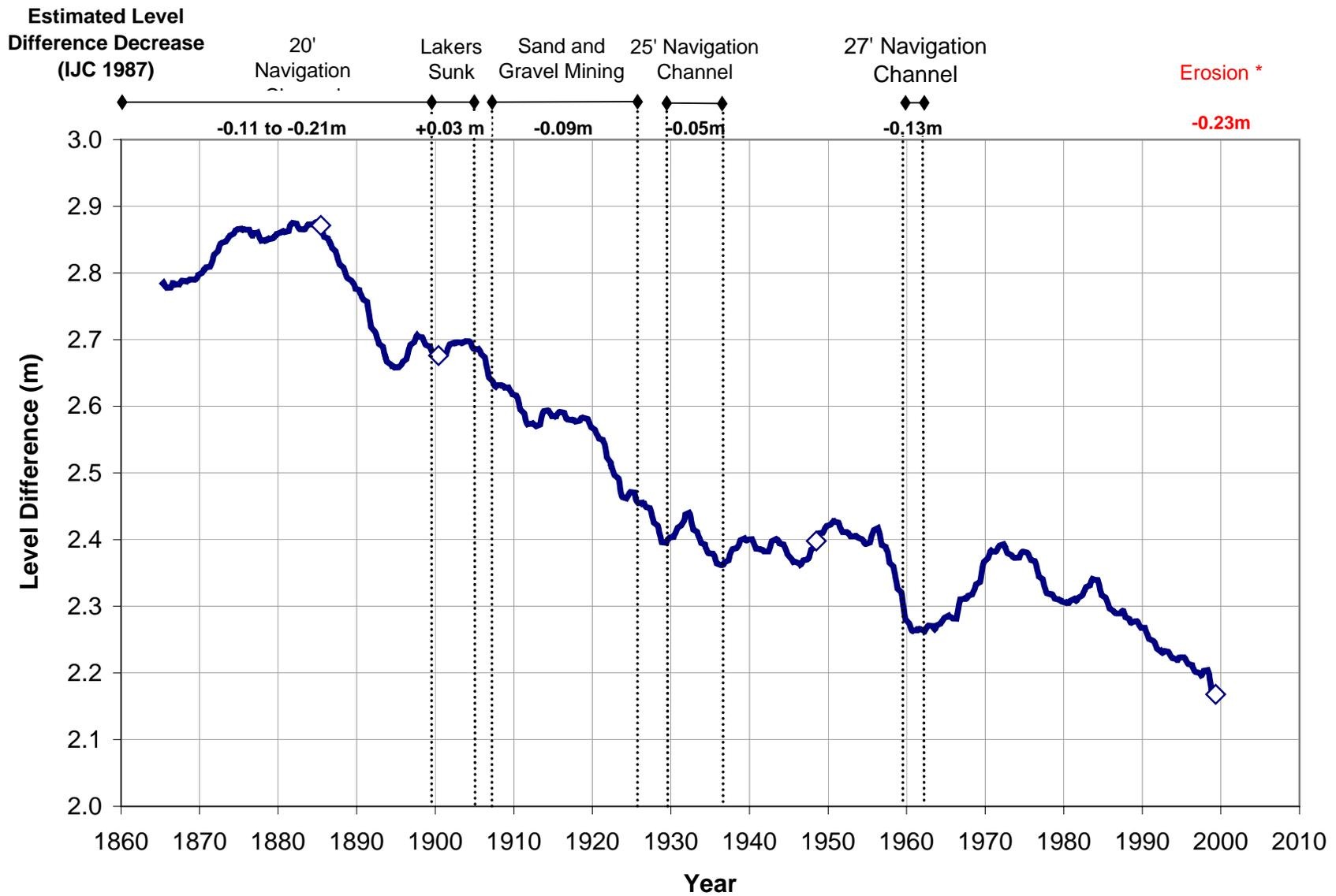
Figure 6.3 Change in Level Difference between Lakes Michigan-Huron and Erie due to Erosion and Man-Made Intervention showing IJC Estimates (seasonal and weather induced changes removed through normalization)
