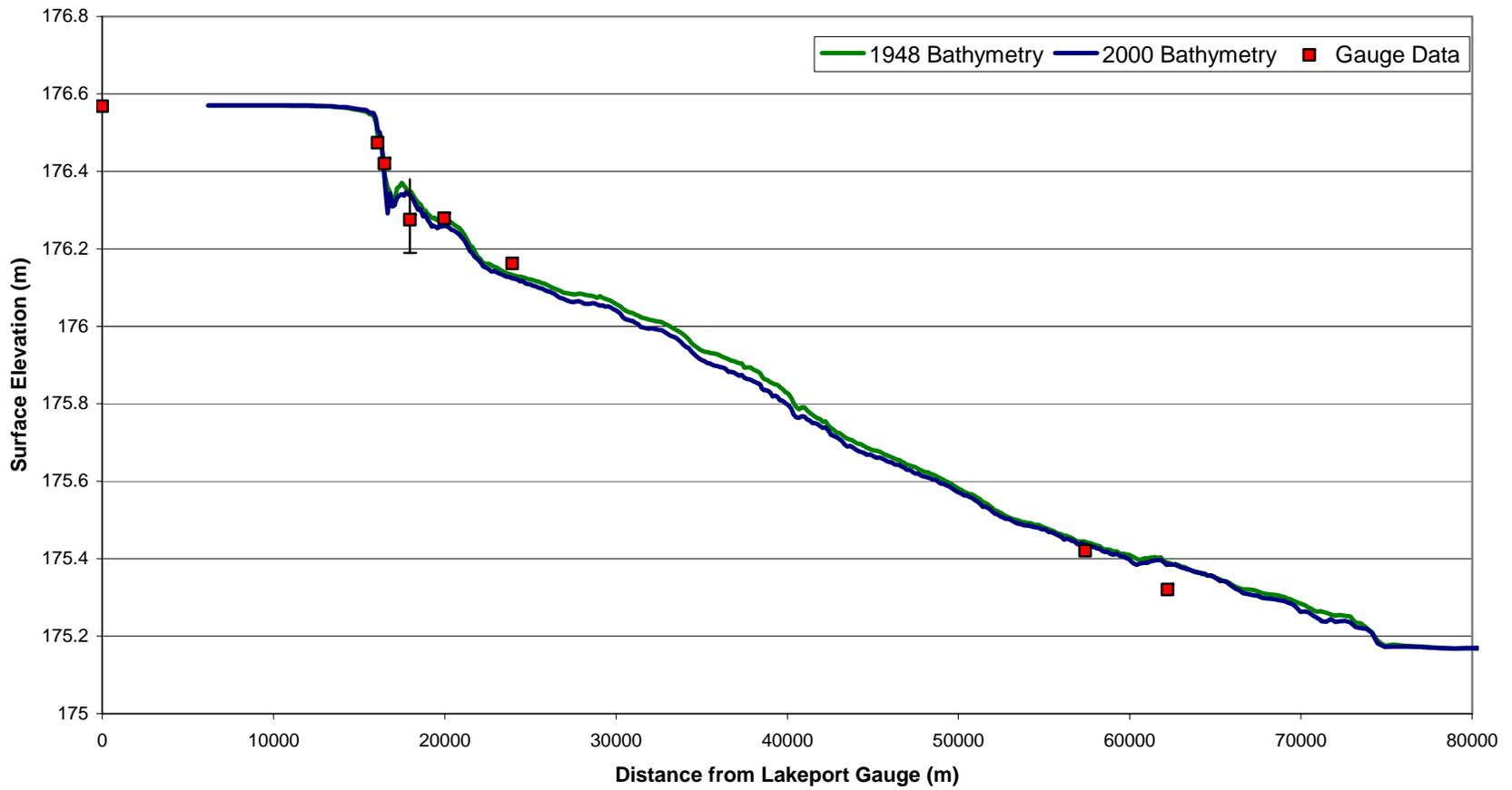
Figure 5.2 Comparison of Model Output with Gauge Data for Mean Lake Levels during August 1968
