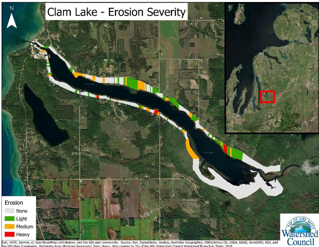
Figure 13 Erosion severity around Clam Lake shoreline
